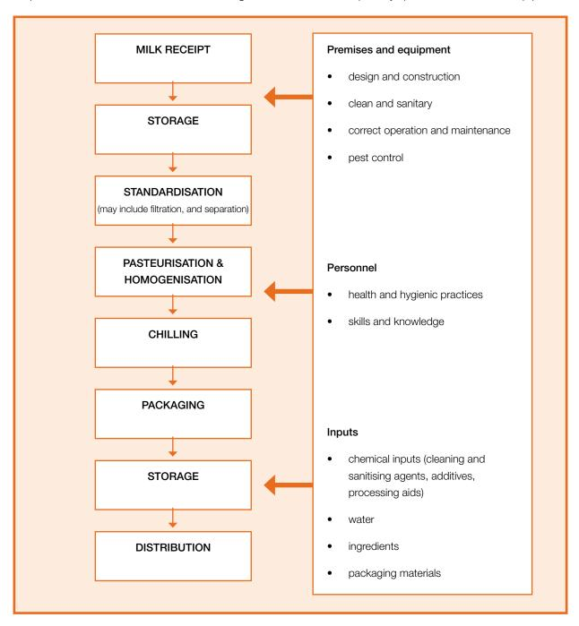
Figure 1: Key steps involved in packaged milk processing
